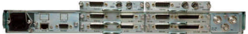
Back panel of CDM-Qx - Depicts multiple configuration options
