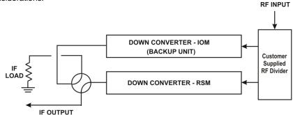
1:1 Redundant Configuration Diagram - Single Source IF Output RSM-XX Installed
