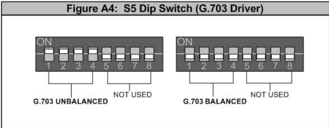
**Figure A4. DIP Switch on the G.703 Driver**
