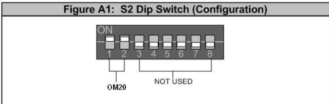
Figure A-1. DIP Switch Positions for the OM20
