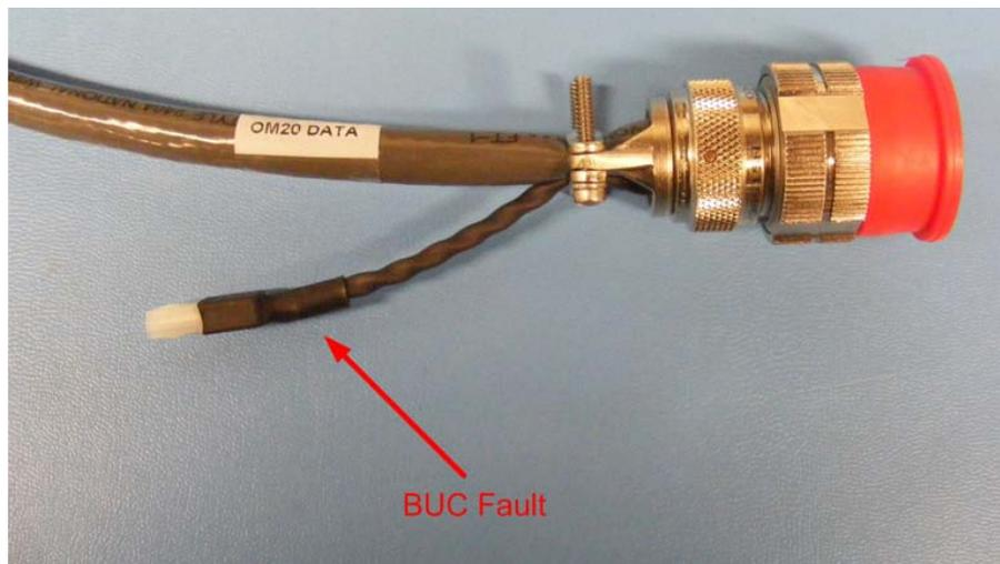
**Figure 5-2 External BUC fault detection on CAR5902 or CAR5918**
