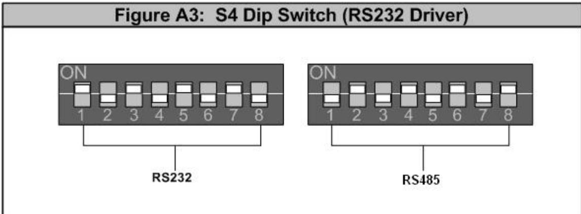
**Figure A3. DIP Switch on the RS232 Driver**
