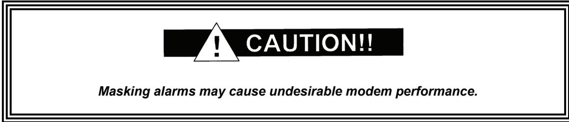
When an alarm is masked, the Front Panel LEDs and the Fault Relays do not get asserted, but the Alarm will still be displayed. This feature is very helpful during debugging or to lock out a failure of which the user is already aware.
