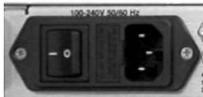
A standard Type 'IEC' detachable, non-locking, 3-prong power cord supplies the Alternating Current (AC) power to the modem.
