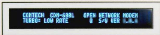
The CDM-600/600L features a **V**acuum **F**luorescent **D**isplay (VFD). The VFD is an active display showing two lines of 40 characters each. It produces a blue light, the brightness of which can be controlled
