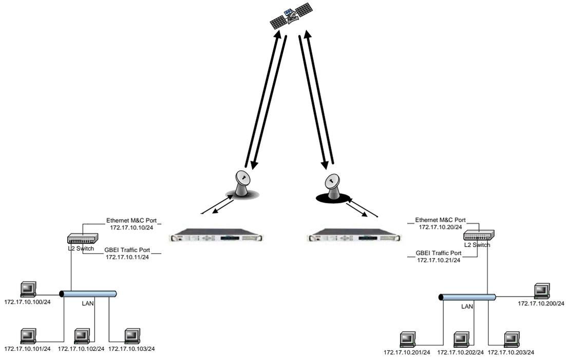
**Figure E-4. Example of GBEI Interface Bridging a Remote Host on a Common LAN over the Satellite**
