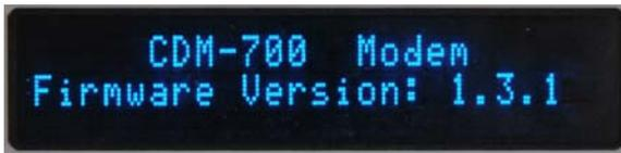
The CDM-700 features a Vacuum Fluorescent Display (VFD). The VFD is an active display showing two lines of 24 characters each. It produces a blue light, the brightness of which can be adjusted. Compared to a Liquid Crystal
