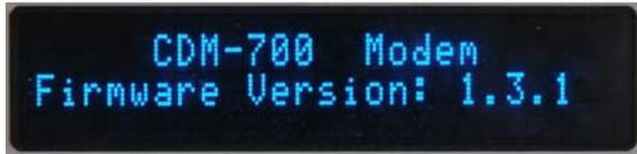
The opening ‘welcome screen’ shown here is representative of what displays whenever power is first applied to the unit (the Firmware Version may differ). Pressing any key displays the top-level **Select** menu.
