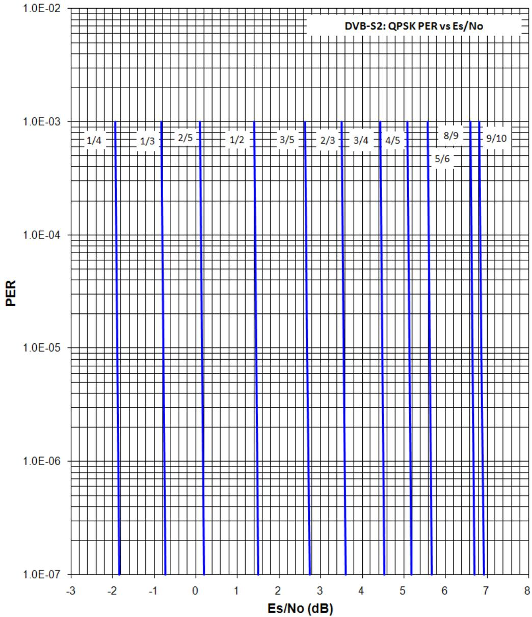
**Figure B-1. DVB-S2 QPSK Packet Error Rate versus Es/No**
