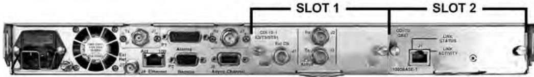
**Figure E-2. CDM-710G/L Rear Panel Data Interface Slots**
