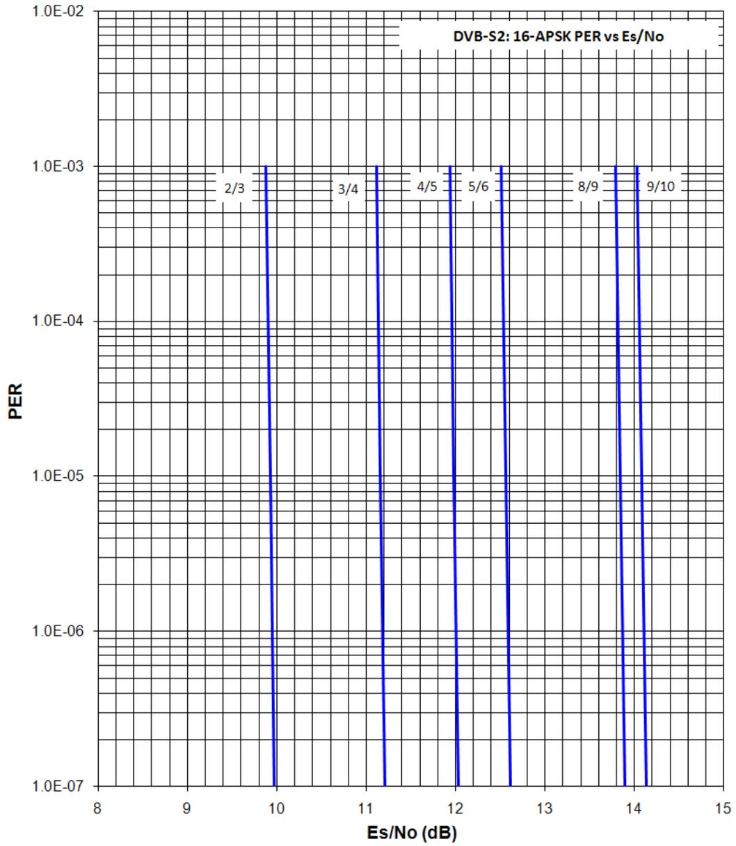
Figure B-3. DVB-S2 16APSK Packet Error Rate versus Es/No
