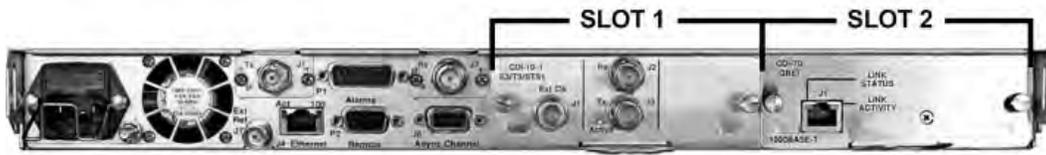
**Figure 1-2. CDM-710G/L Rear Panel Data Interface Slots**
