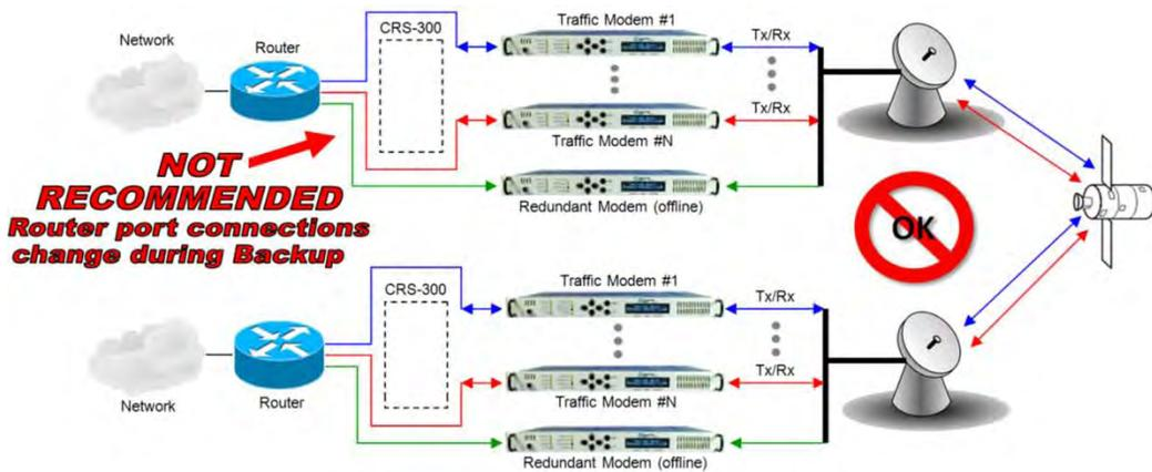
Figure A-6. Wired-around for Hub-to-Hub with Standard Traffic using Routers
