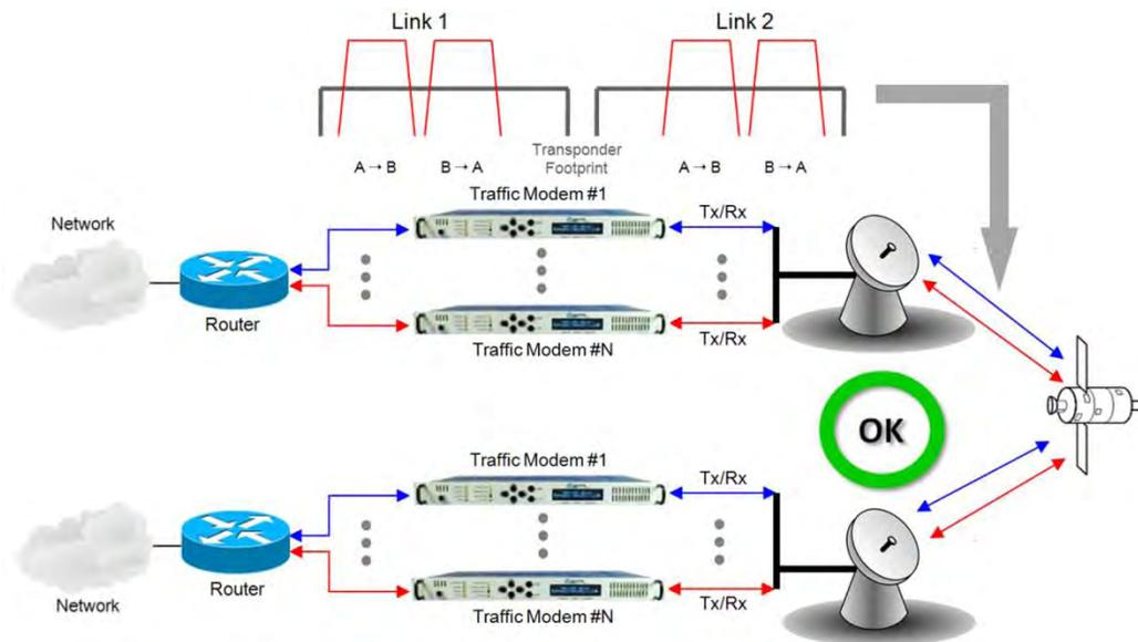
**Figure A-4. Hub-to-Hub with Standard Traffic using Routers**
