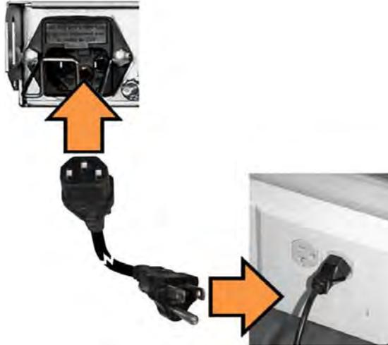
**Figure 4-7. Apply AC Power to the Unit**
