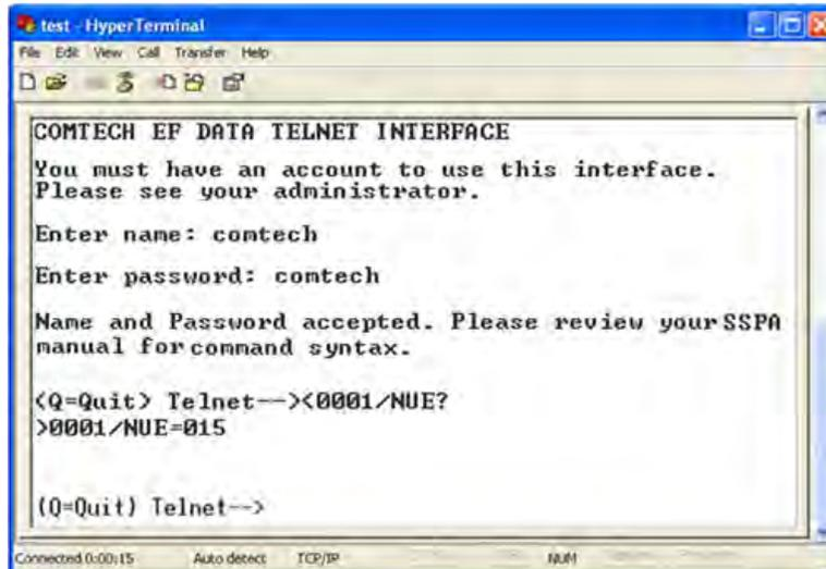
**Figure 8-2. Telnet Interface Example – HyperTerminal**
