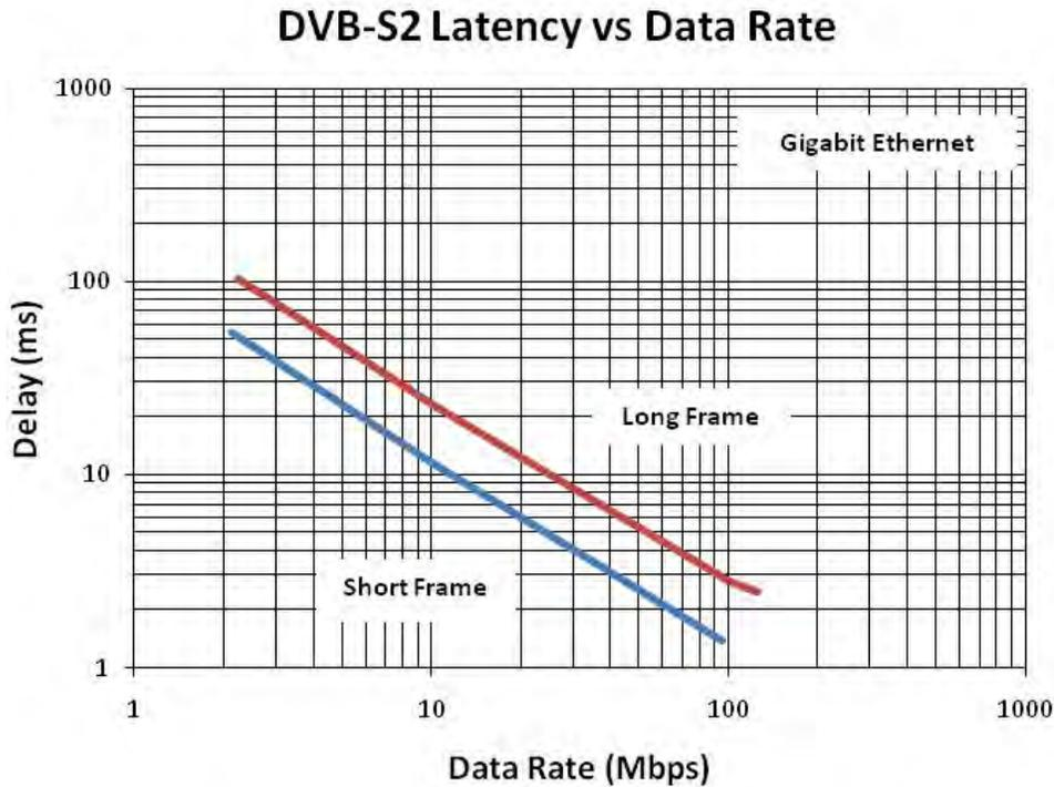
Figure B-5. CDM-710G/L Gigabit Ethernet Latency with Modem in IF Loopback
