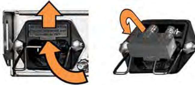
**Figure 4-6. Replace the AC Fuses**
