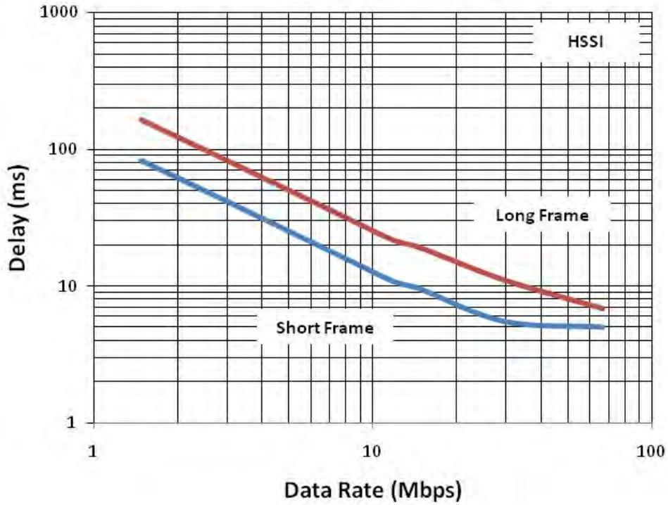
Figure B-6. CDM-710G/LHSSI Latency with Modem in IF Loopback
