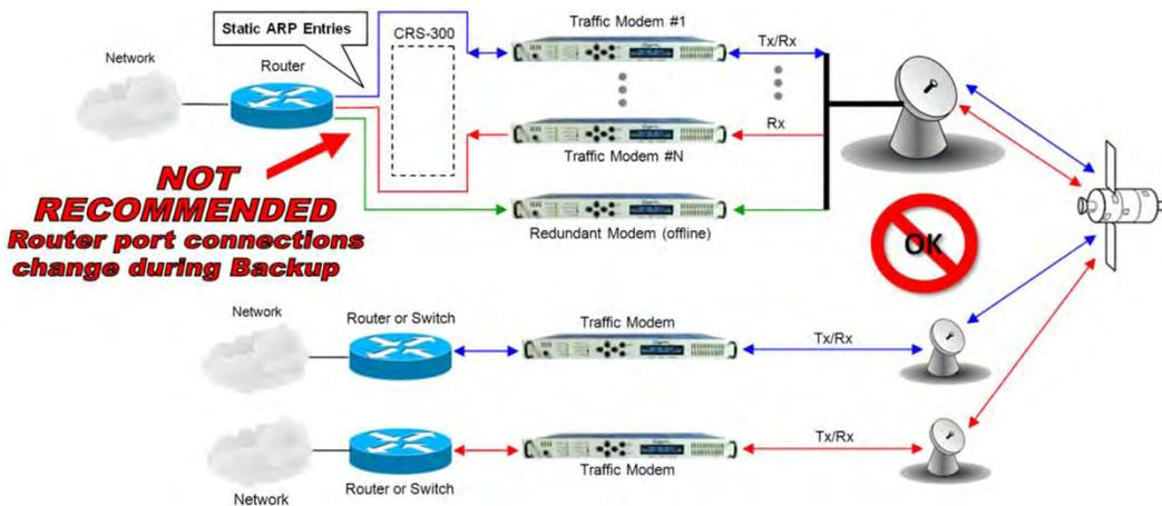
**Figure A-12. Wired-around for Point-to-Multipoint with Routers**
