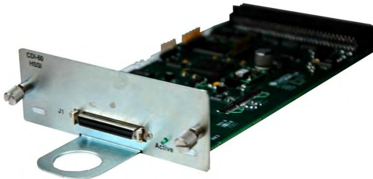
Figure D-1. CDI-60 HSSI Data Interface Module
