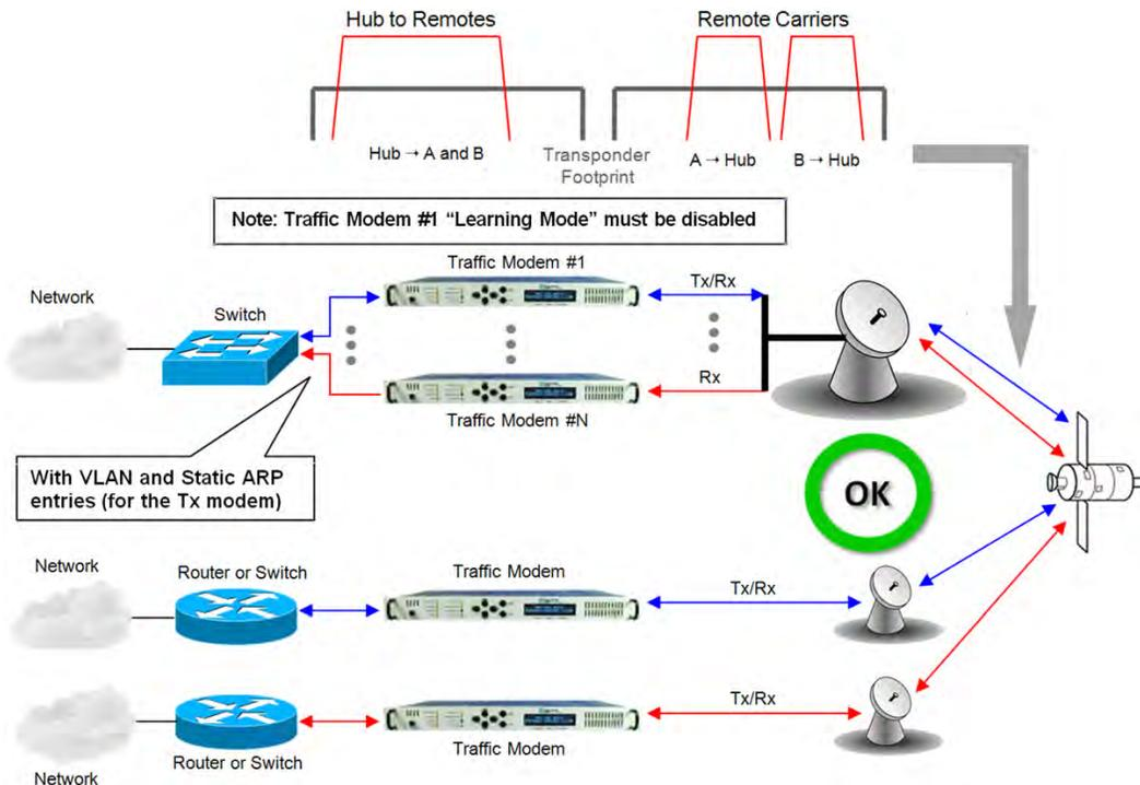
**Figure A-13. Point-to-Multipoint using Switches**
