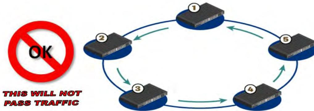
**Figure A-1. Networking Loop with Switches**
