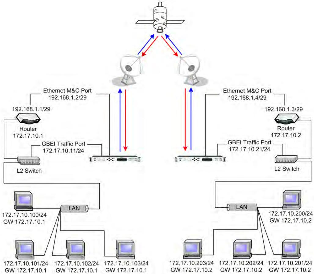
**Figure E-6. M&C Port Assignment Example: IP Address NOT on Common LAN**
