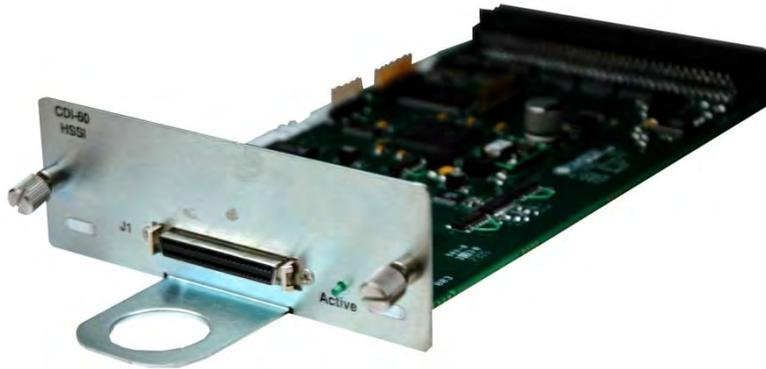
**Figure F-5. CDI-60 HSSI Data Interface Module**
