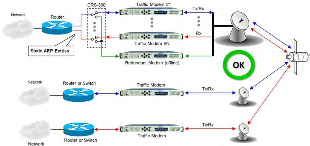
**Figure A-11. Wired-thru for Point-to-Multipoint with Routers**
