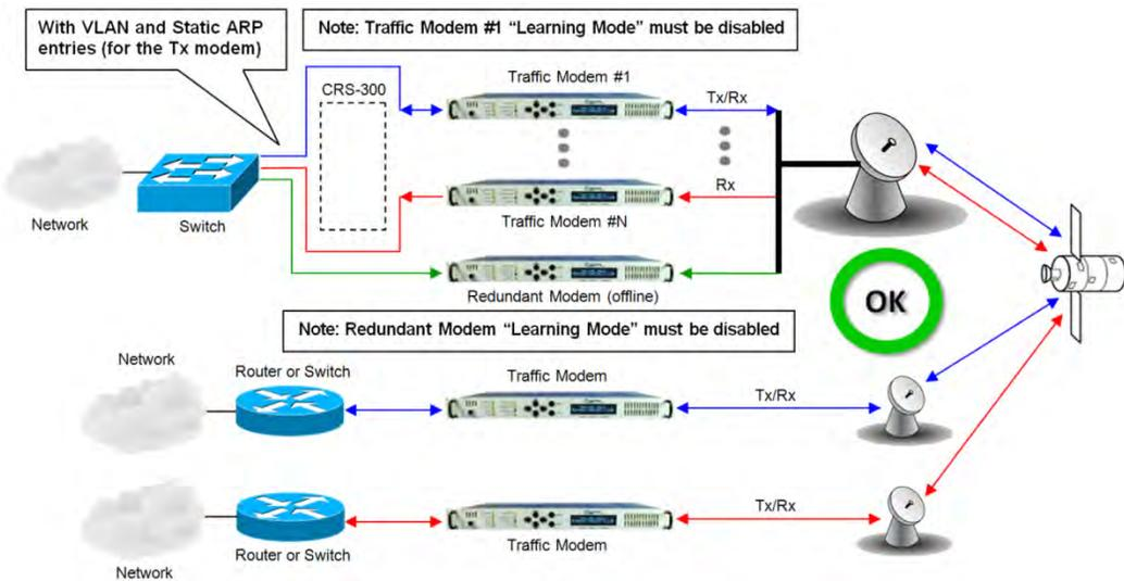
**Figure A-15. Wired-around, Hub-to-Remotes, Split-path Traffic using Switches (Point-to-Multipoint)**
