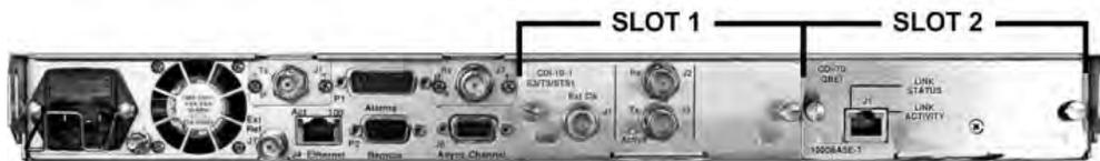
**Figure F-1. CDM-710G/L Rear Panel Data Interface Slots**
