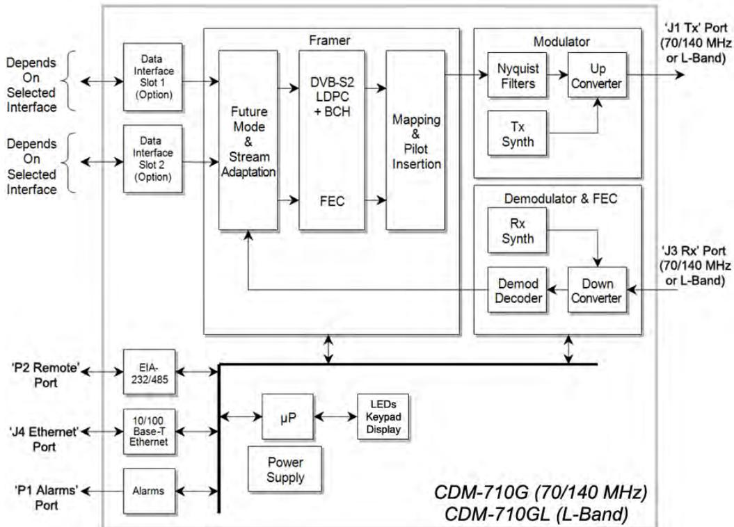
**Figure 1-3. CDM-710G/L Block Diagram**
