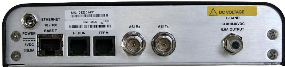
Figure 3-1. Digicast Media Router S2 Receiver – Rear Panel
