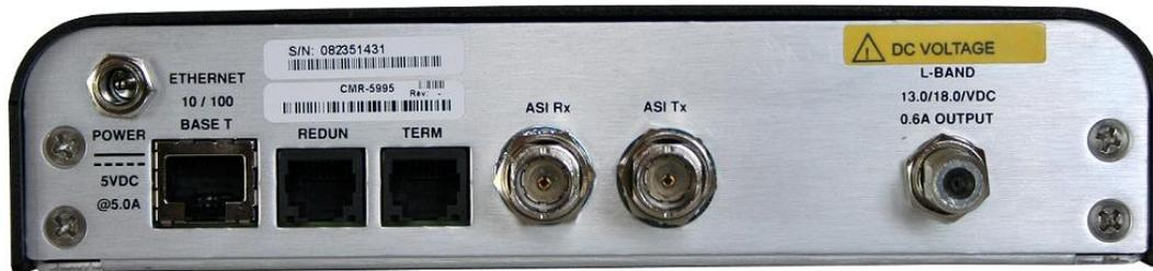
**Figure 1-2. Digicast Media Router S2 Receiver – Rear Panel**
