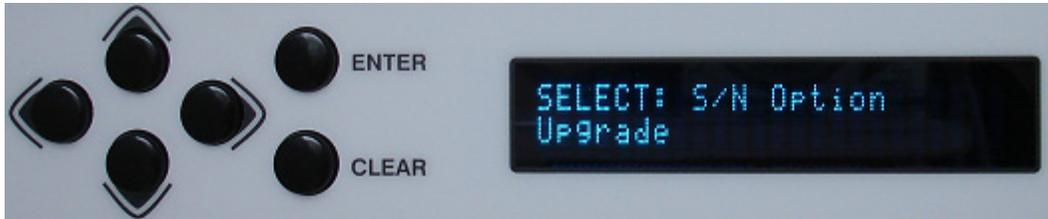
Comtech EF Data’s FAST (Fully Accessible System Topology) system permits the purchase and installation of options through special authorization codes, entered remotely or through the front panel. FAST allows immediate implementation of different options through the user interface keypad. All FAST options are available through the basic platform unit.
