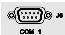
The **J6 COM 1** connector is a 9-pin Type ‘D’ female (DB-9F) connector that provides the EIA-232/EIA-485 Interface. The pinout specifications are provided in **Table 3-6**.
