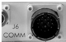
The **J6 COMM** connector, featured on both the BUC-4000 Block Up Converter and BDC-4000 Block Down Converter Modules, is used for connecting the module to the MBT-4000 Base Module **J3 UNIT 1 COMM** or **J6 UNIT 2 COMM** connectors via the 15-15 Power & Signal Harness (CEFD P/N CA/WR10963-1), as shown in **Figure 3-2** and **Figure 3-3**.
