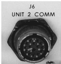
The **J6 UNIT 2 COMM** connector is used for connecting the MBT-4000 Base Module Unit 2 section to the **J6 COMM** connector featured on both the BUC-4000 Block Up Converter and BDC-4000 Block Down Converter Modules, via the 15-15 Power & Signal Harness (CEFD P/N CA/WR10963-1), as shown in **Figure 3-3**.
