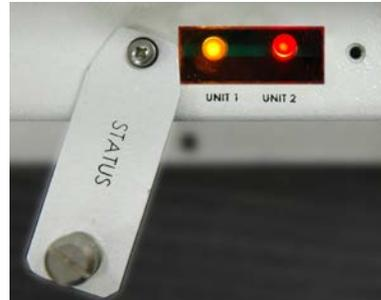
**Figure B-2. Faulted System Example**
