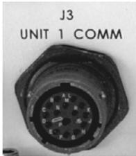
The **J3 UNIT 1 COMM** connector is used for connecting the MBT-4000 Base Module Unit 1 section to the **J6 COMM** connector featured on both the BUC-4000 Block Up Converter and BDC-4000 Block Down Converter Modules via the 15-15 Power & Signal Harness (CEFD P/N CA/WR10963-1), as shown in **Figure 3-2**.
