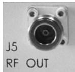
The **J5 RF OUT** connector, located on the BUC-4000 Block Up Converter Module, is a Type 'N' female connector, used to provide the upconverted RF Output.
