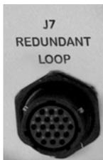
The **J7 REDUNDANT LOOP** connector is used to connect the MBT-4000 Base Module, via the Redundant Loop Bus Cable (CEFD P/N CA/WR11224), to another base unit for a dual base (redundant) setup.
