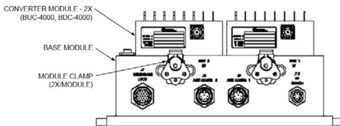
The Base Module for the MBT-4000 system – which provides the M&C, Power Supply, and Reference interfaces – may be located near or on the antenna. Guide pins and mechanical clamps keep the band-specific BUC and BDC modules in place on top of the Base Module.
