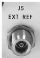
The **J5 EXT REF** connector is a Type 'N' female connector, used to provide an External 10MHz Reference Input.
