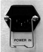
A standard, detachable, non-locking, 3-prong power cord (IEC plug) supplies the Alternating Current (AC) power to the converter.
