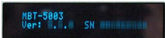
The MBT-5003 features a **Vacuum Fluorescent Display (VFD)**. The VFD is an active display showing two lines of 24 characters each. It produces a blue light, the brightness of which
