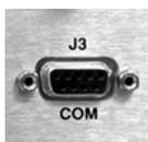
The **J3 | COM** EIA-485 4-wire interface is a 9-pin type ‘D’ (DB-9F) connector (the mating connector is a DB-9M connector). The pinout specifications for EIA-485 are contained in **Table 3-2**.
