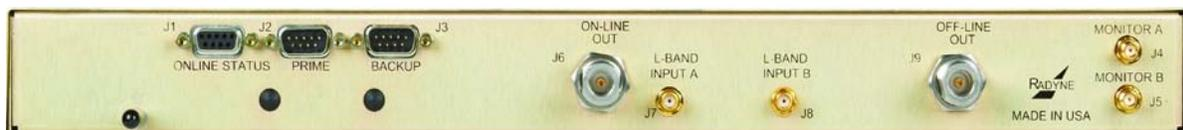
Figure 1-4 RRS11-L L-band Solid-State Transfer Switch (Rear Panel)
